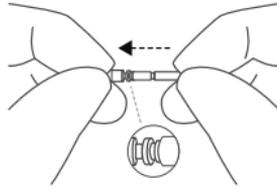
2. Gently press the replacement tip straight into the sound outlet until the outer ring lies flush with the sound outlet.
