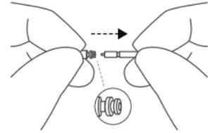
3. Pull the tool straight out - the new wax guard will remain in place. Please remember to re-attach dome again, or attach a fresh dome.
