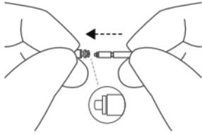
1. Insert the replacement tip of the tool into the sound outlet.
