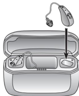
2. Place both hearing aids in the charging bays. Right hearing aid goes into the charging bay marked with a red dot. Left hearing aid goes into the charging bay marked with a blue dot. The receiver goes into the receiver bay.
