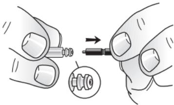
Pull the tool straight out - the new wax guard will remain in place. Please remember to re-attach dome, or a fresh dome.
