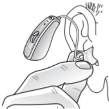
*Slide and twist the earmould all the way into the ear canal.*
