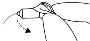
3. Check that the dome is securely mounted by carefully lifting the lower part of the dome and verifying that the collar completely covers the ribbed end of the receiver.
