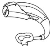
1. Align the tip of your DAI adapter with the groove on top of the battery door.
