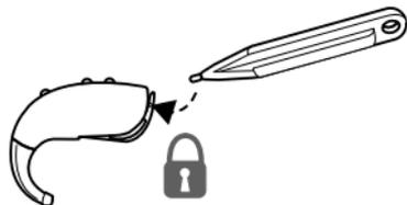
To unlock the battery door simply repeat the same procedure but pushing the slider to the right instead. You can now change the battery as described in How to change the battery.
