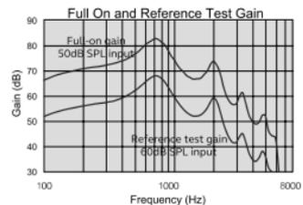
Data in accordance with ANSI S3.22-2014, IEC 60118-0:2015. Measured in a 2cc coupler.
