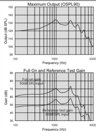
Data in accordance with ANSI S3.22-2014, IEC 60118-0:2015. Measured in a 2cc coupler.
