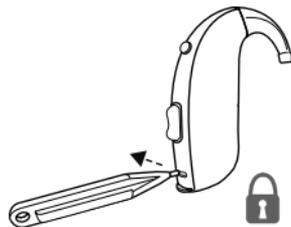
To unlock the battery door simply repeat the same procedure but sliding the lock to the right instead. You can now change the battery as described in How to change the battery.
